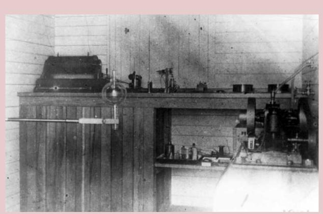
One of New Zealand's early X-ray plants (1904). Note the induction coil (at left on bench) as the 'HT supply'; and the absence of any radiation shielding.
